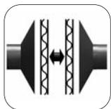
This unique design feature ensures that each case is opened positively from both sides. It ensures the efficient and reliable opening of cases, and overcomes problems that can be associated with stiff board and glue migration from the manufacturer's joint.
