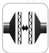
This unique design feature ensures that each case is opened positively from both sides. It ensures the efficient and reliable opening of cases, and overcomes problems that can be associated with stiff board and glue migration from the manufacturer's joint.
