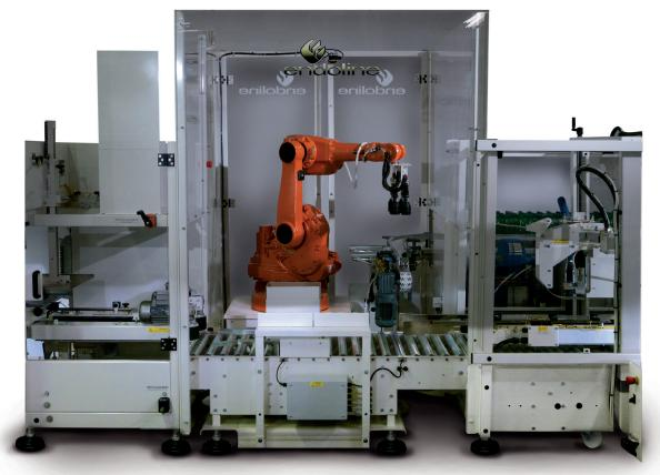
The Endoline 330 series of robotic machines are designed to fully automate the packing of products into cases, trays or crates on new or existing production lines and remove labour intensive operations, which are a major cause of cost and repetitive strain injuries. Its features are aimed specifically at customers seeking efficiency through simplicity in terms of set-up, operation and maintenance, which makes the 330 series a particularly cost effective investment.
