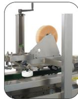
Our unique four column design provides added stability for the taping bridge to ensure the machine runs smoothly at all times with minimal interruption and it provides the support necessary for the floating bridge feature. This fully automatic machine is fitted with two pairs of columns for additional support to the folding section.
