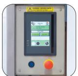
Our digital message display unit allows for rapid set-up, entering of case data and machine status. Simple mechanical operation and clear access allows for easy cleaning and maintenance.
