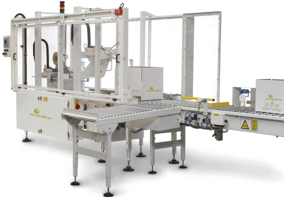
This is the dominant machine of its type having originally been developed for the biscuits and snack foods industries. It automatically adjusts to random sizes while sealing small and large, lightweight and heavy cases without the need for an operator. It is fully automatic and provides secure and accurate taping at speeds of up to 20 cases per minute. Fully automatic random sealing machines are ideally suited to applications where there is insufficient room for a sealer on each packing line.
