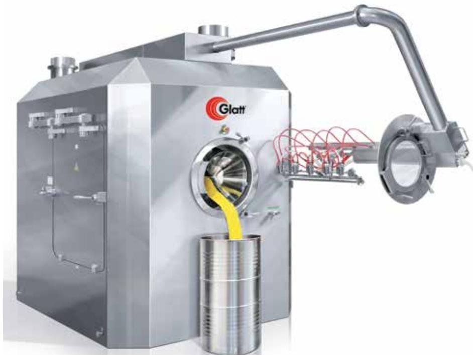
Open front discharging using the SmartScoop® discharging system
