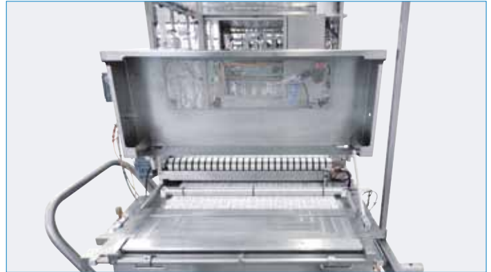
Lidding system: on the ground to easy maintenance and quickly change of the reel of paper
