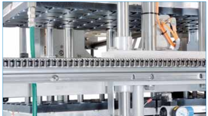
Lidding system: on the ground to easy maintenance and quickly change of the reel of paper
