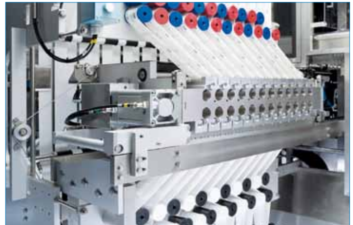
Extractible unit for label introduction. Limited floor space
