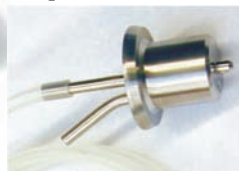
Spray nozzle for binder addition
