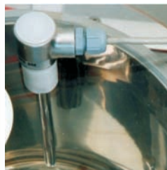
Measurement of product temperature
