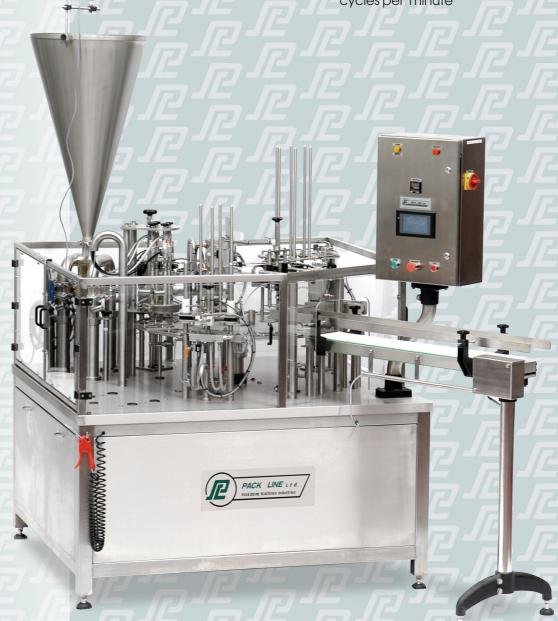
The NBM is the technologically advanced line of the Pack Line Fully Automatic Rotary Filling and Sealing machines with smooth indexor driven movement of 12-positions rotary platform. It makes the NBM machines the best solution for liquids, as well as for paste, granulated and powdered products, Dairy products, salads and dressings, sweet desserts, cosmetics and much more is the short list of products which can be filled by those machines.
